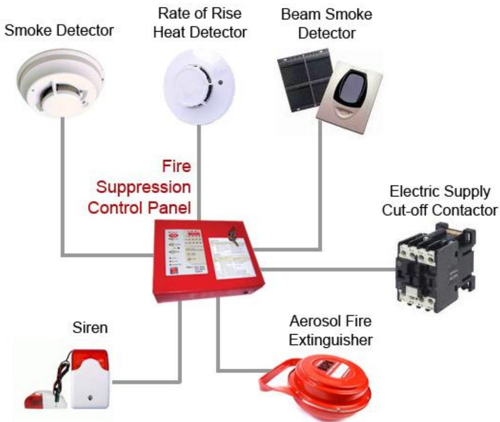
Above diagram shows the schematic of the whole system. Aerosol is released as soon as one of the sensors is activated. One can connect various types of detectors for Smoke, Heat, Flame, Flammable gases etc. The Fire Suppression system monitors the status of the sensors and activates output devices like Sounder, Suppression agent etc.
