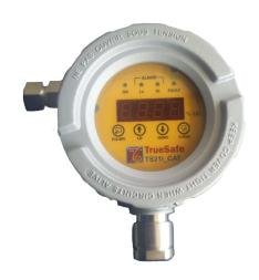
Relay output is provided and this output can be connected to the conventional Gas Detection Panel OR SCADA system. For BMS connectivity detector has provided RS485 output. Additionally 4-20mA and Selectable 0-5 V & 0-10V Analog output could be also available. Enclosure used is suitable for Zone 1 & Zone 2 hazardous areas.
